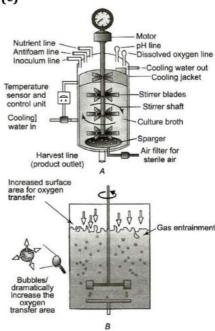
A-Simple stirred-tank bioreactor for continuous
