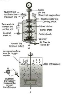
A-Simple stirred-tank bioreactor for continuous culture.
